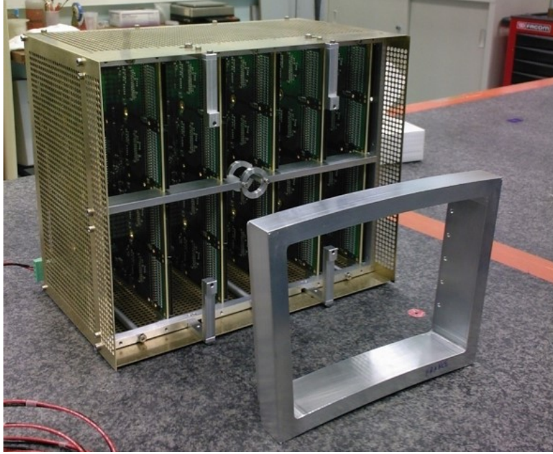
Figure 5.8: Original T2K electronics with light shielding in from of a mechanical frame.
