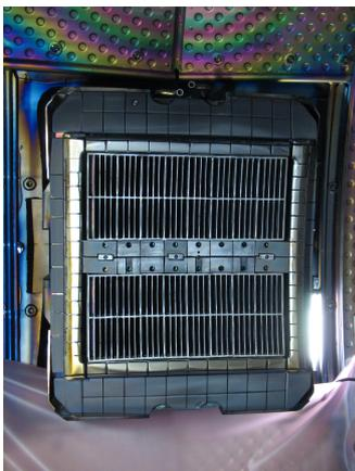
**Figure 5.3:** Tore Supra Multijunction launcher C2 as view from inside the vacuum vessel. (128 waveguides, total dimensions 50 x 40 cm, 1989). Frequency: 3.7GHz.
