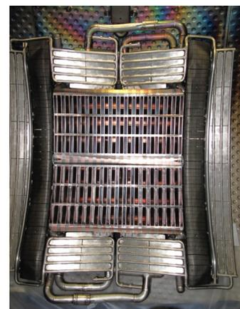
**Figure 5.6:** The WEST PAM antenna LH2. (96 active waveguides, 102 passive waveguides, approx. 7 tons, front face dimensions 60cm x 60cm, 3.7 GHz, 2009).
