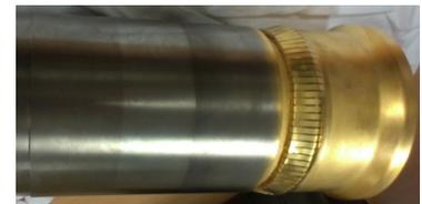
**Figure 4.28:** RF Contact prototype tested in 2014.
