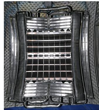
**Figure 5.4:** Tore Supra Multijunction launcher LH1 (288 waveguides, total dimensions 60cm x 60cm, 1999). Frequency: 3.7GHz.
