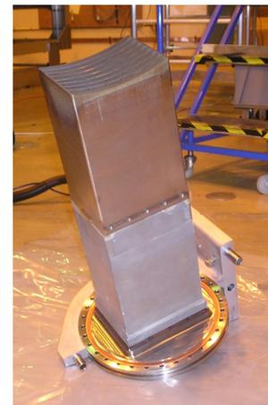
**Figure 5.1:** Picture of the grill mouth of the COMPASS-D LH launcher, made of 8 waveguides. Generator frequency was 1.3 GHz. 165x82mm Rectangular waveguides.
