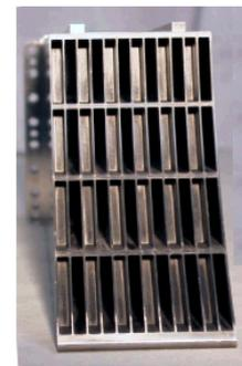
**Figure 5.5:** PAM prototype tested on the FTU tokamak (24 active waveguides, 24 passive waveguides, 8 GHz, 2003) [257, 258].
