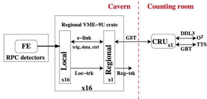
Figure 4.8: Schematic of the MID readout electronics architecture [226].
