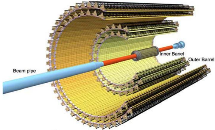
Figure 4.4: Layout of the new ITS detector [227].
