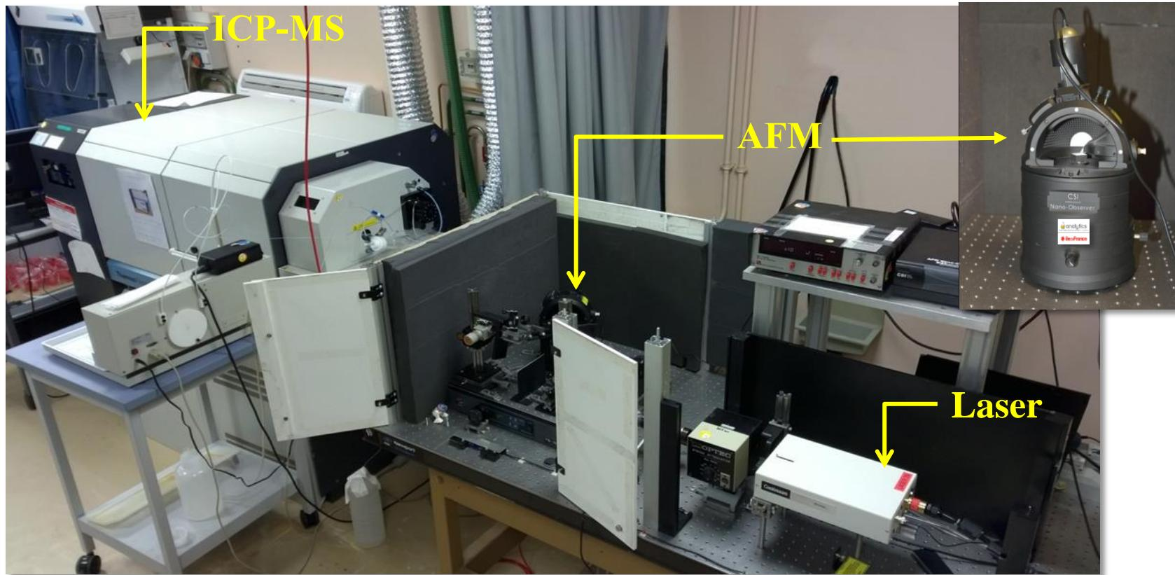
*Laser Nd:YAG (266 nm) , pulse duration 4 ns.*
