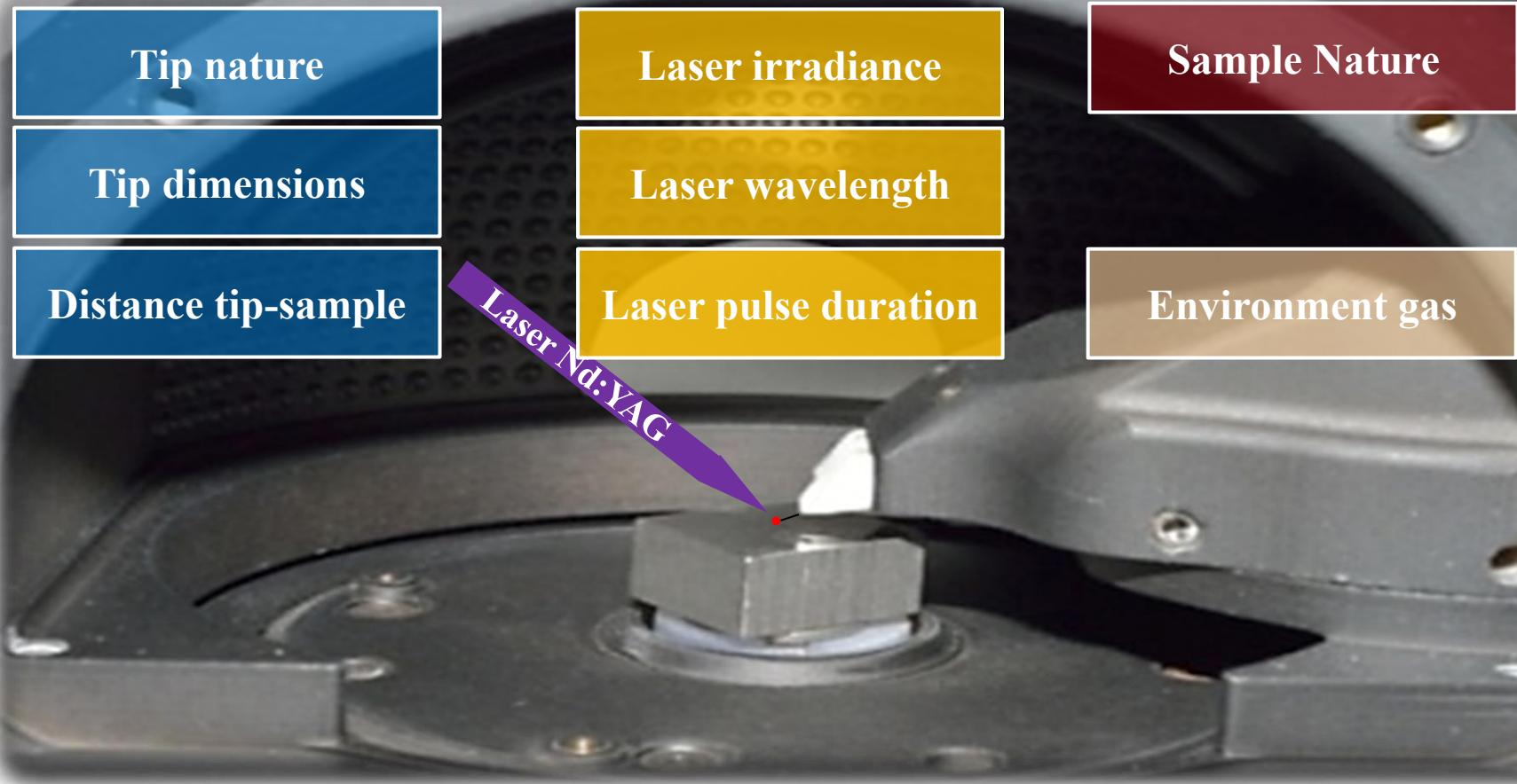
Parameters influencing the near field ablation efficiency, resolution, craters dimensions (amount of ablated mass)
