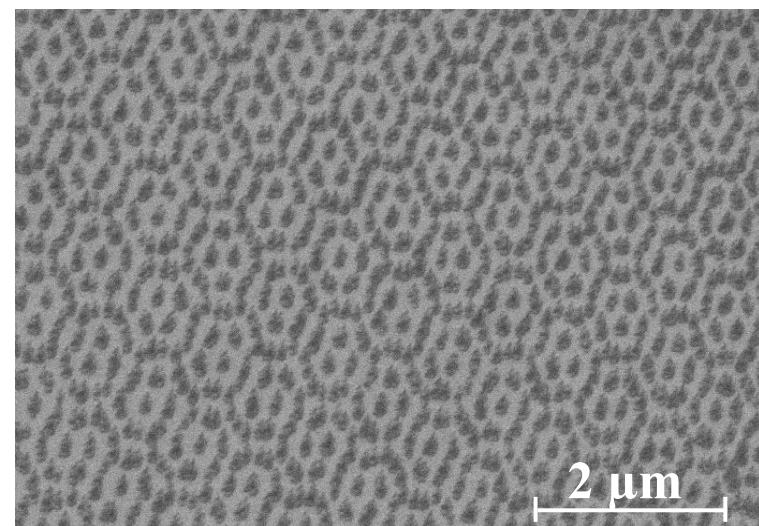
The diameter of the obtained craters ranged from 100 to 120 nm using a single laser pulse.
