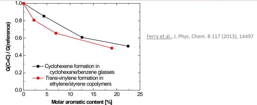
Double bonds formation in cyclohexane/benzene organic glasses and in ethylene/styrene copolymers irradiated using ion beam at 11 K under vacuum
