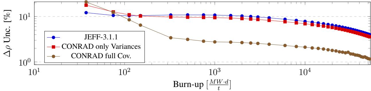
**Figure 8.** Relative reactivity loss uncertainty as a function of the burn-up for the JHR. The propagation of JEFF-3.1.1  $U^{235}(n_{th}, f)$  FY uncertainties on the reactivity loss is compared to what we obtained from FY uncertainties generated by CONRAD, with and without correlations.
