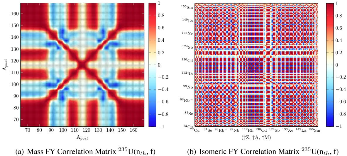
**Figure 2.** Correlation matrices for mass (left) and isomeric (right) fission product yields for the thermal fission of  $^{235}\text{U}$ . Only FY greater than  $10^{-7}$  have been considered and ordered in ascending charge, mass and isomeric state.
