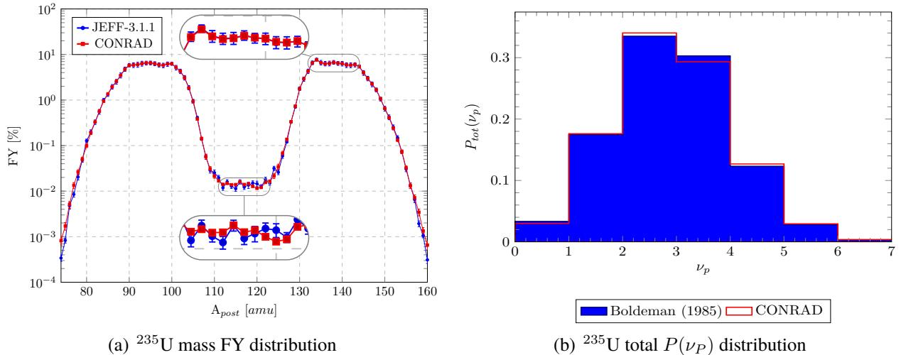
**Figure 1.** Comparison between JEFF-3.1.1 and CONRAD mass FY distribution for  $^{235}\text{U}(n_{th}, f)$  (left). FY model parameters adjusted by CONRAD can also represent quite well experimental data on the total prompt neutron emission probability (right).
