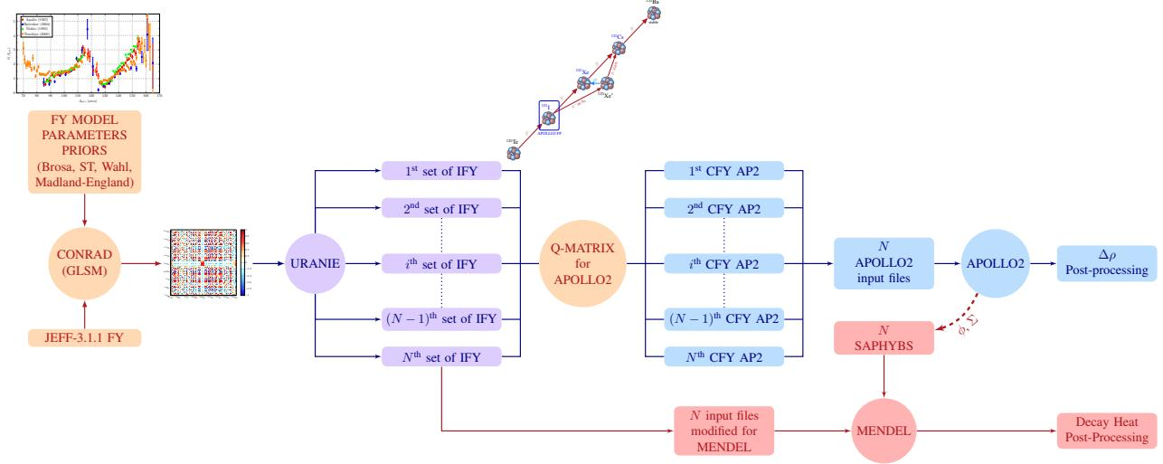
**Figure 4.** Monte Carlo error propagation flow chart for reactivity and decay heat uncertainty estimation using URANIE. With IFY we indicated independent fission yields, on the other hand we called CFY the cumulative ones.
