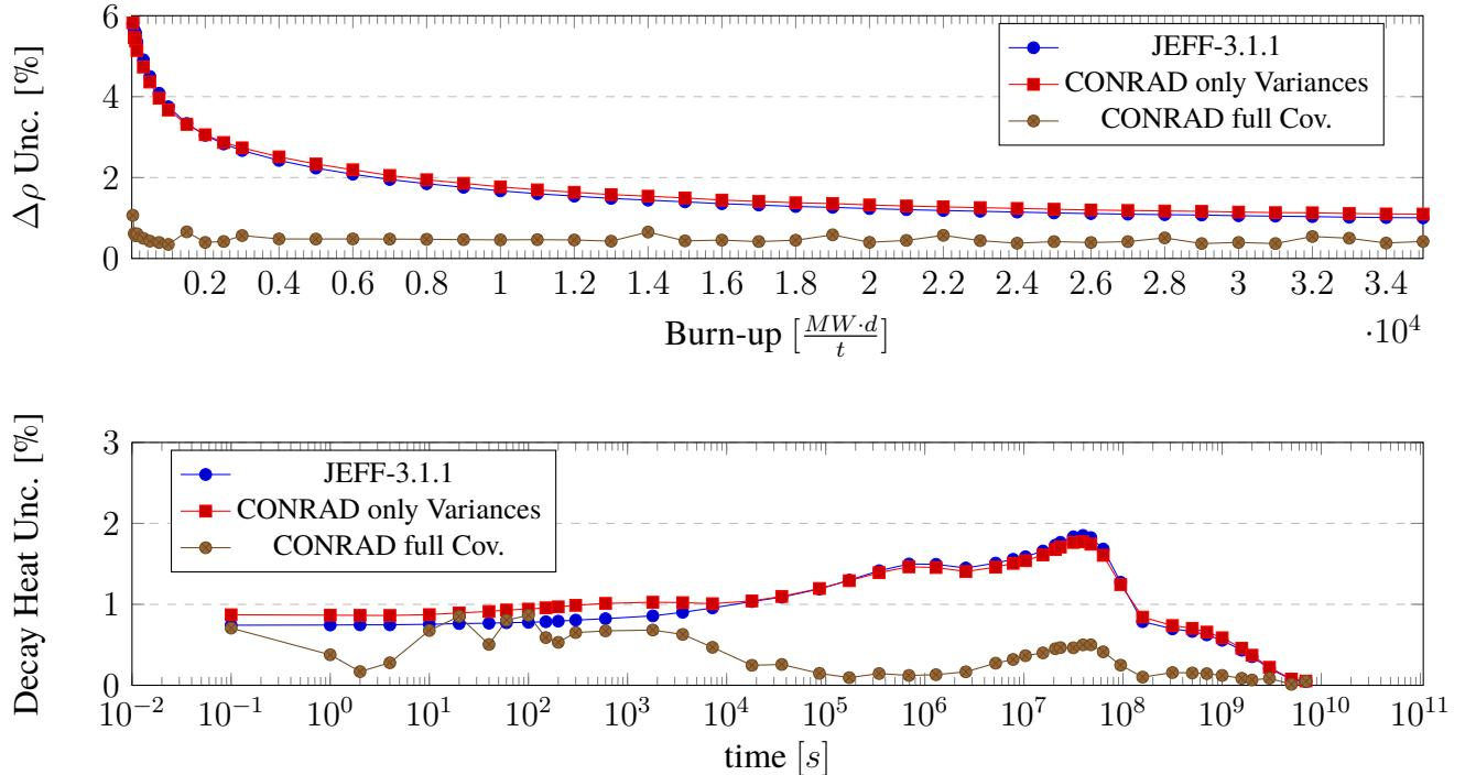
**Figure 6.** Reactivity loss (top) and decay heat (bottom) uncertainties for a PWR-MOX pin-cell. The propagation of JEFF-3.1.1 Pu<sup>239</sup>(n<sub>th</sub>, f) FY uncertainties is compared to what we obtained from FY uncertainties generated by CONRAD, with and without correlations.
