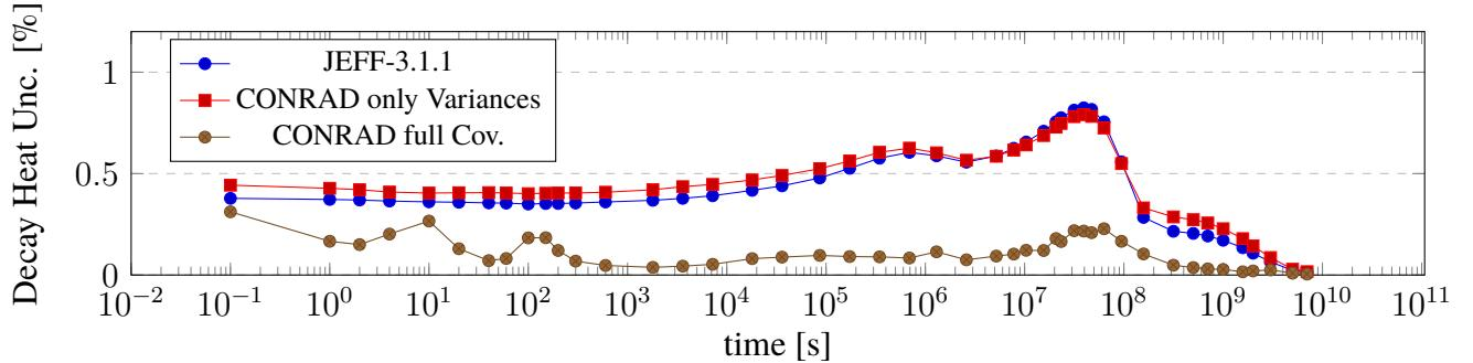
**Figure 7.** Decay heat uncertainty for a PWR-MOX pin-cell. The propagation of JEFF-3.1.1 <sup>241</sup>Pu(n<sub>th</sub>, f) FY uncertainties on the decay heat is compared to what we obtained from FY uncertainties generated by CONRAD, with and without correlations.
