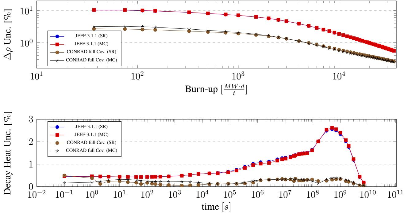
**Figure 5.** Reactivity loss (top) and decay heat (bottom) uncertainties for a UOX-PWR pin-cell. The propagation of JEFF-3.1.1  $U^{235}(n_{th}, f)$  FY uncertainties using a simple sandwich rule (SR) and the Monte Carlo propagation (MC) has been compared to what we obtained from FY uncertainties generated by CONRAD including correlations.
