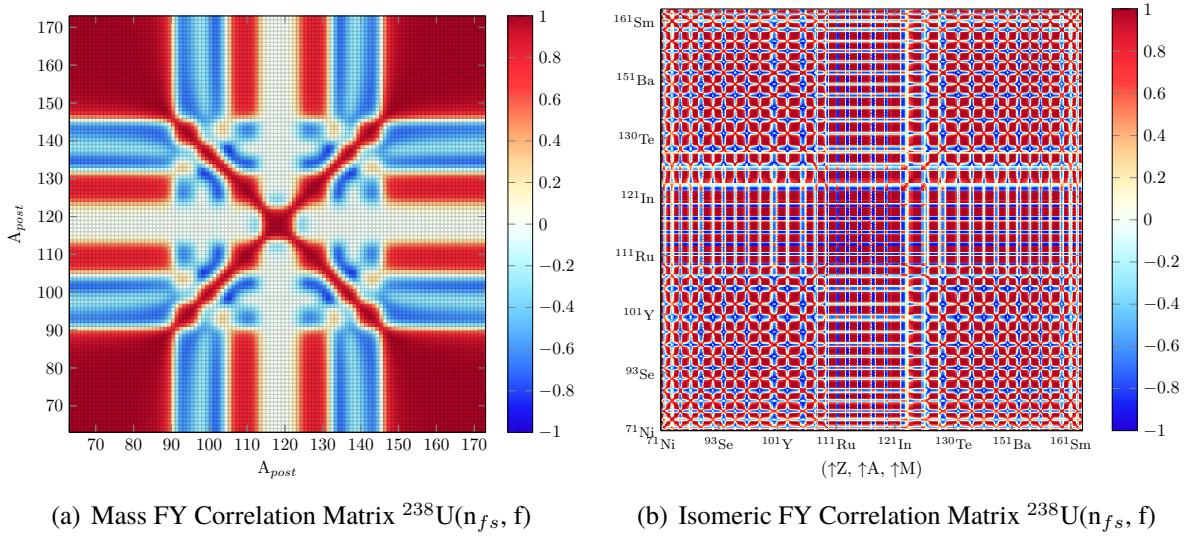
**Figure 3.** Correlation matrices for mass (left) and isomeric (right) fission product yields for the fast fission of  $^{238}\text{U}$ . Only FY greater than  $10^{-7}$  have been considered and ordered in ascending charge, mass and isomeric state.
