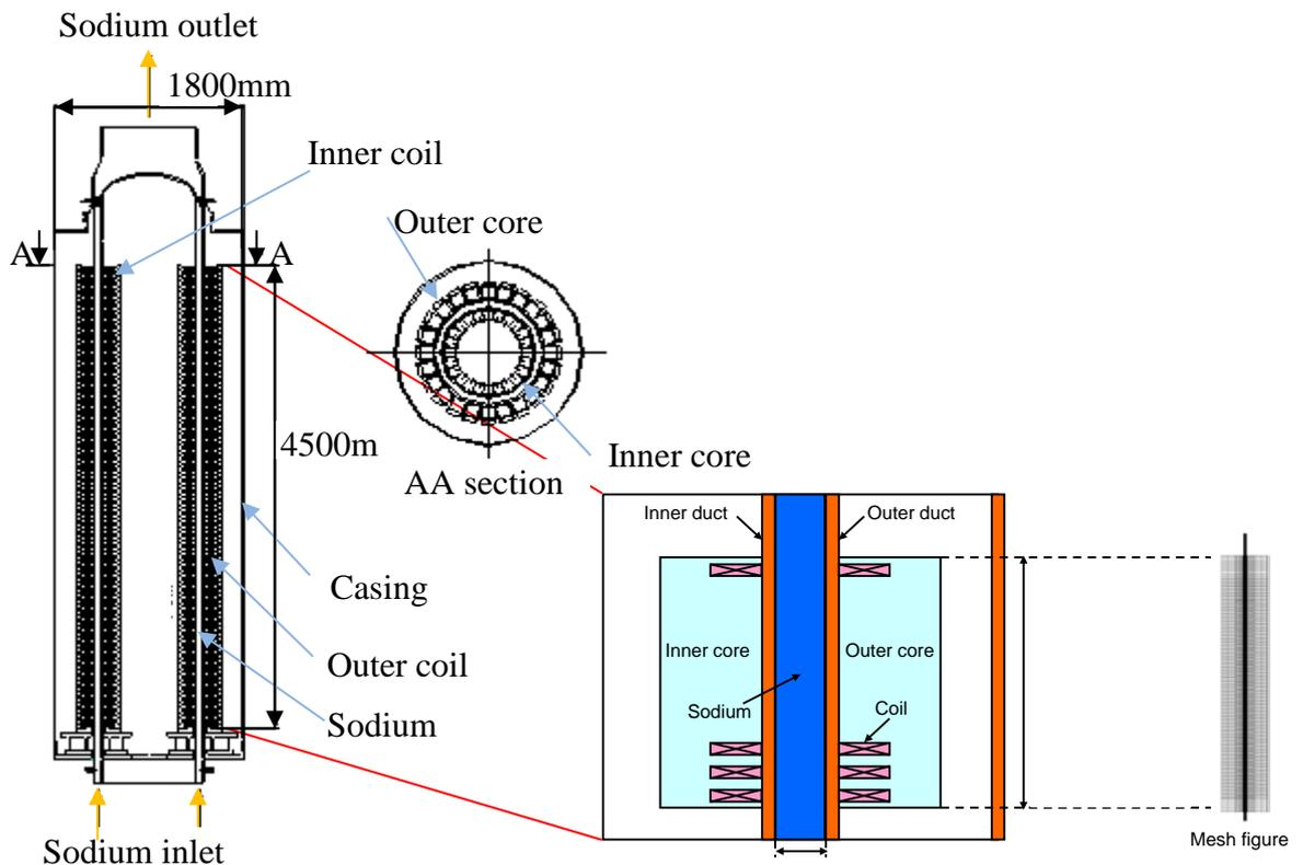
**Figure 3:** Electromagnetic fluid analysis two-dimensional axis-symmetrical model
