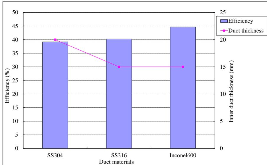
**Figure 2:** Compare result of the duct materials
