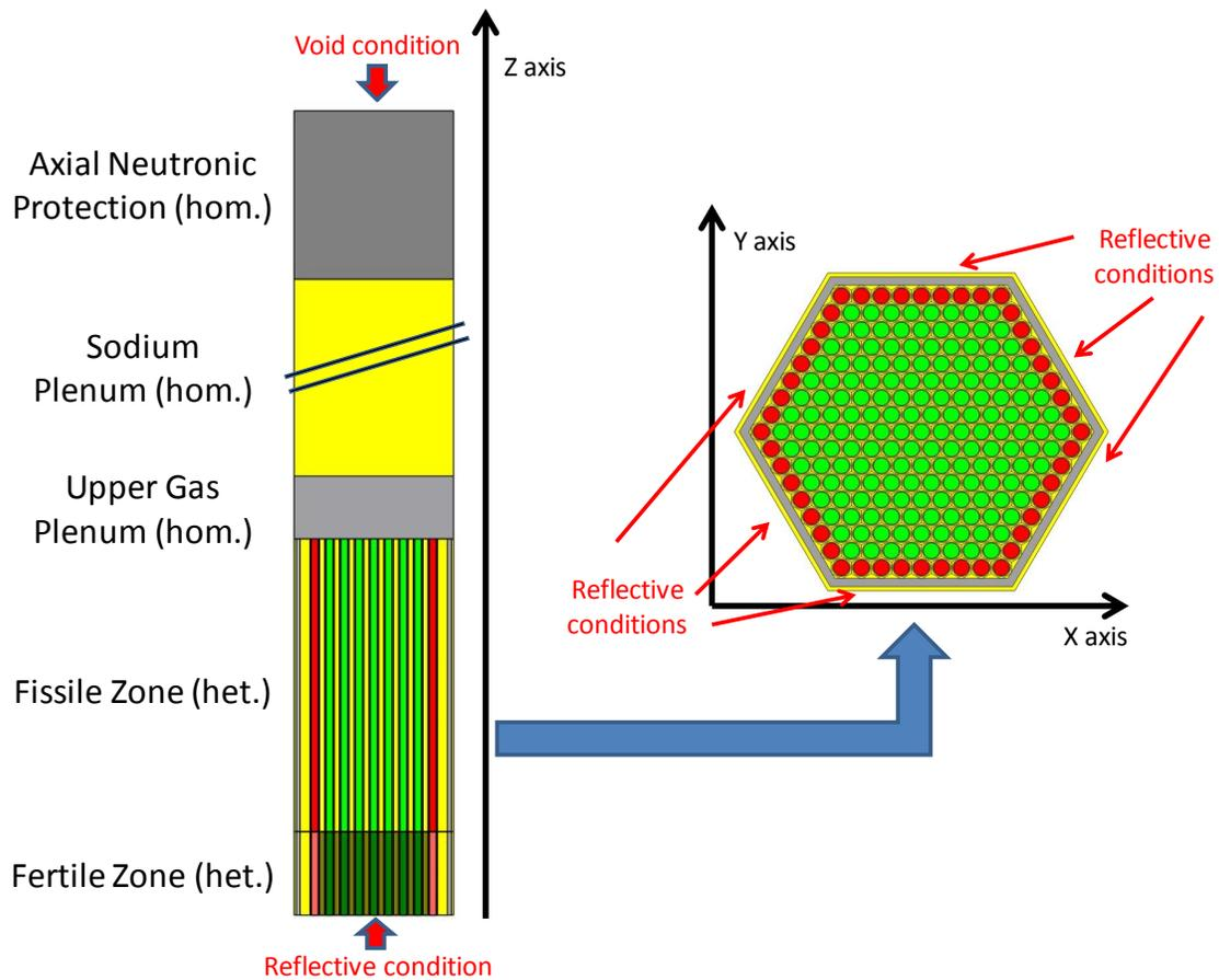
**Figure 2.** Geometry of the Upper Half 3D Inner Fuel Sub-Assembly of the CFV. Five different axial zones are detailed (from bottom to top): fertile, fissile, gas plenum, sodium plenum and neutronic protection. Only the fertile and fissile zones are described explicitly, the other zones are composed of homogenized media.
