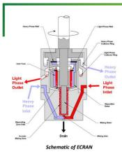
Aqueous and organic phases are fed at the bottom of the mixing zone by means of two channels. They are pumped by the mixing rotor and flow into the annular region between the mixing rotor and the stationary cylinder where they are mixed by shearing.
