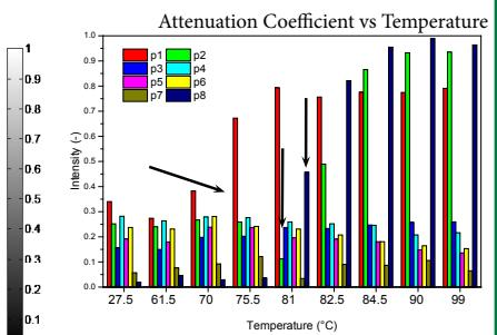
Main changes of attenuation coefficient take place at the edge of the sample
