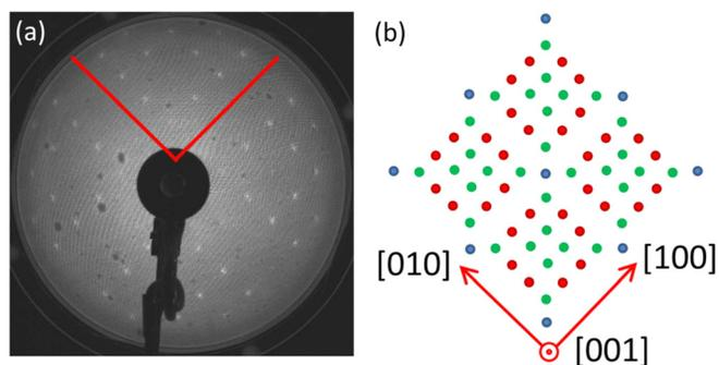
FIG. 2. (a) LEED image on SBN(001) single crystal surfaces at 45 eV. (b) Schematic LEED diffraction pattern showing superposition of two patterns,  $(\sqrt{5} \times \sqrt{5})R26.6^\circ$  (red) and  $(5\sqrt{2} \times \sqrt{2})R45^\circ$  (green). The common points are marked by blue color.
