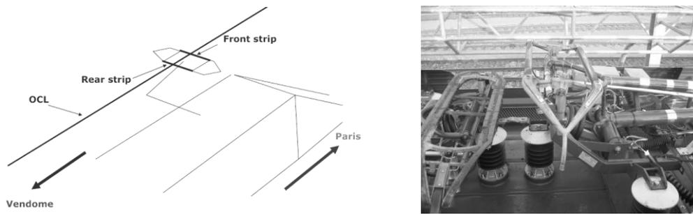
Figure 4. Pantograph configuration for Paris-Vendôme TGV field tests.
