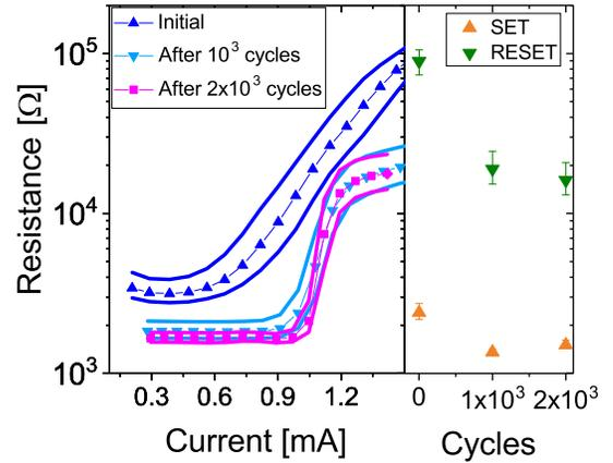
**Fig. 8.** Left: R-I characteristic at the beginning of the devices life and after endurance for TiTe/GST. Right: 4 kb TiTe/GST SET and RESET resistances evolution along cycles performed with pulses of 10  $\mu$ s to accelerate and evidence the evolution.
