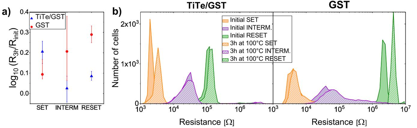
**Fig. 7.** Data retention evaluated after annealing at 100°C for the SET, intermediate and RESET states in TiTe/GST and GST 4 kb arrays. a) The resistance drift is quantified as the ratio between the resistance measured after a 3 hours annealing and the initial resistance. Median values and variability are represented. b) Resistance distributions of the three states before and after 3 hours annealing at 100°C.
