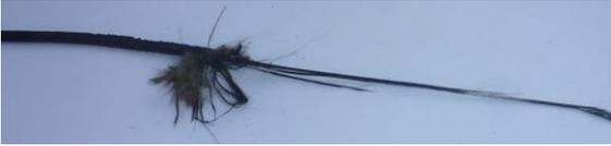
Fig. 3. Typical aspect of the security cable after more than two hours at 750°C.
