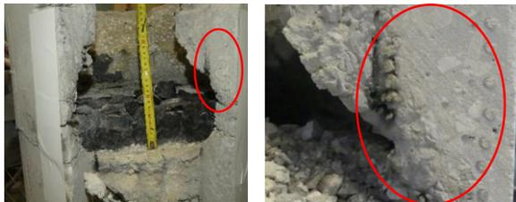
Fig. 22. *Post-mortem* analysis with remaining sensing cables apparently intact.
