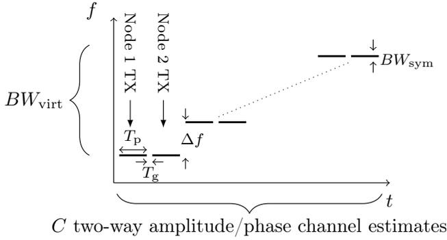
Fig. 1. Multi-channel ranging signaling process for  $C$  sequentially aggregated narrowband ( $BW_{\text{syms}}$ ) channels.
