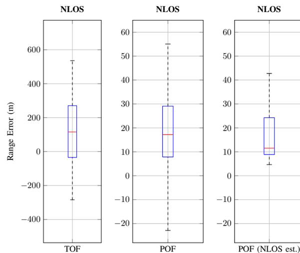
Fig. 7. Performance comparison for NLOS reference points
