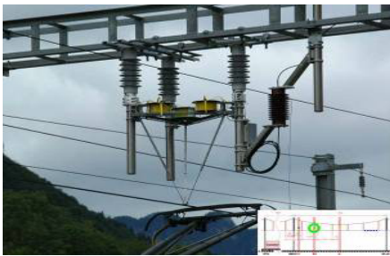
Fig. 2a: FBG-based tripod for 3D displacement sensing
