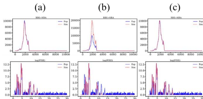
**Figure 3.** Unknown and predicted NRA and PIXE spectra of  $\text{TiC}_{0.5}\text{O}_{0.5}$  compound with (a) high density meshing (b) low density meshing (c) low density meshing + data augmentation
