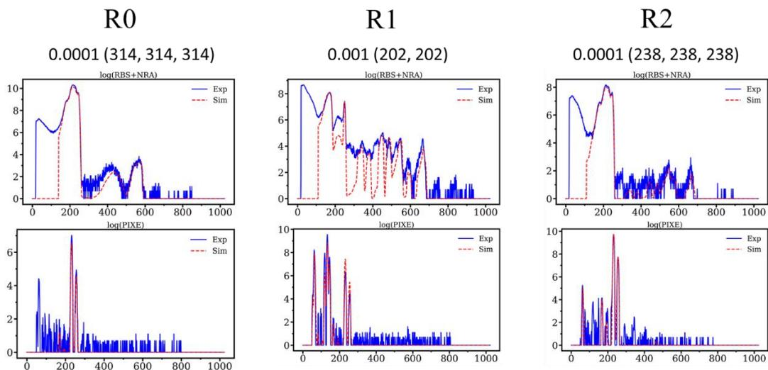
**Figure 6.** Unknown and predicted NRA and PIXE spectra for the 3 identified regions from Fig1b. Neural network hyperparameters are indicated for each phase.
