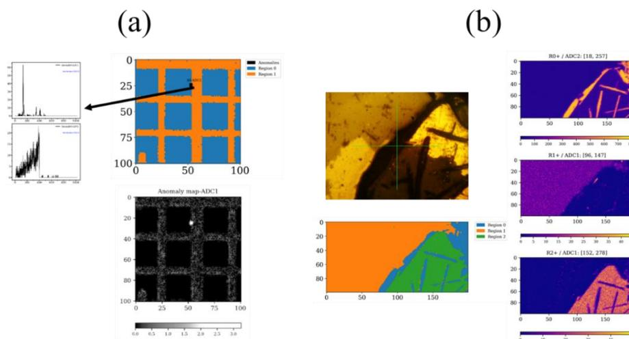
**Figure 1.** Hyperspectral data processing from (a) a copper grid (b) a multiphasic sample. Anomaly map (a, bottom) highlights a mineral dust. Chemical maps from the multiphasic sample are shown on the right.
