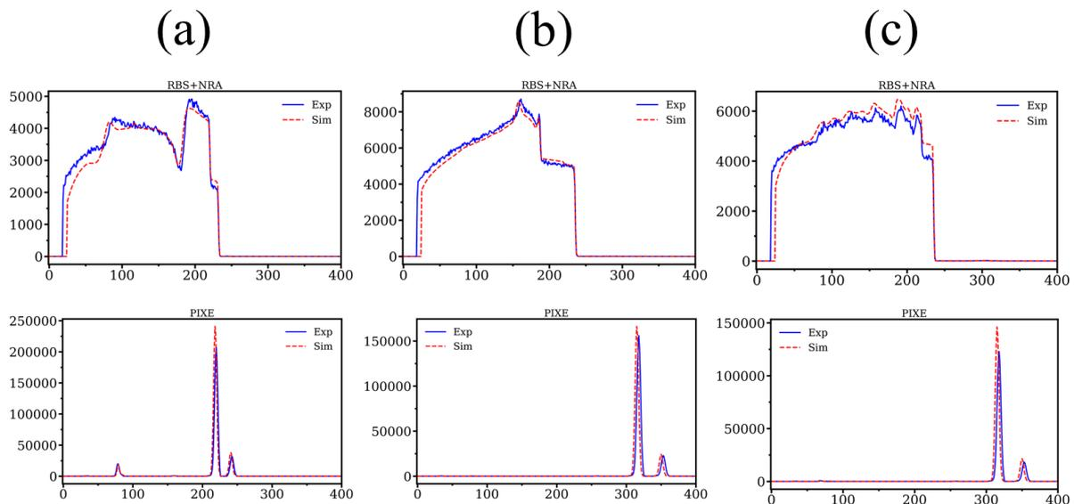
**Figure 4.** Experimental and predicted RBS and PIXE spectra for (a) FeS<sub>2</sub>, (b) GaN (c) GaP from an ANN trained with Ga, N, P, Fe and S
