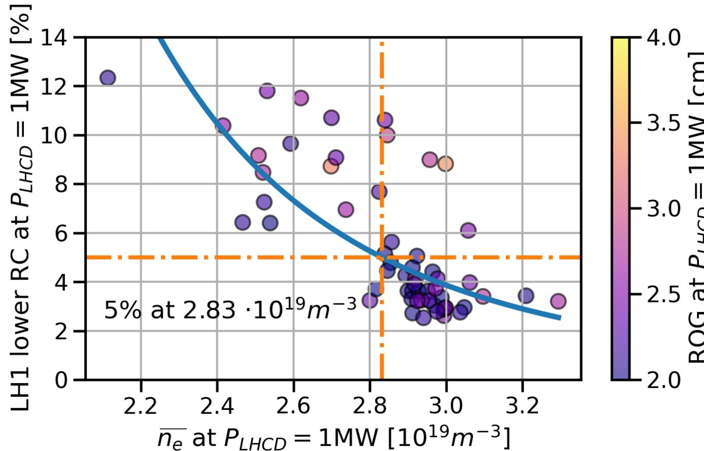
Reflection coefficient on lower LH1 antenna modules
