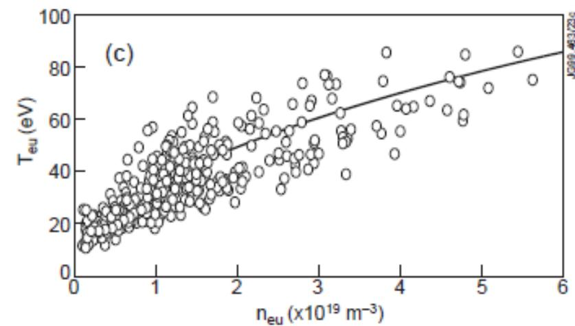
**Figure 2.** (a)  $T_{eu}$  versus  $n_{eu}$  for separatrix values: OSM results for the JET Mark II divertor, H mode. A sin-
