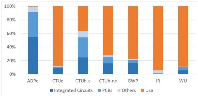
Fig. 3. LCA results of the transmitter antenna. 100% represents the complete life cycle (manufacturing + use). “Others” category is composed of connectors, solders, resistors and capacitors.
