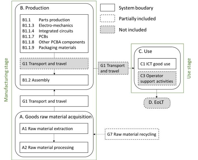
Fig. 2. System boundaries according to ITU L.1410 standard [15].
