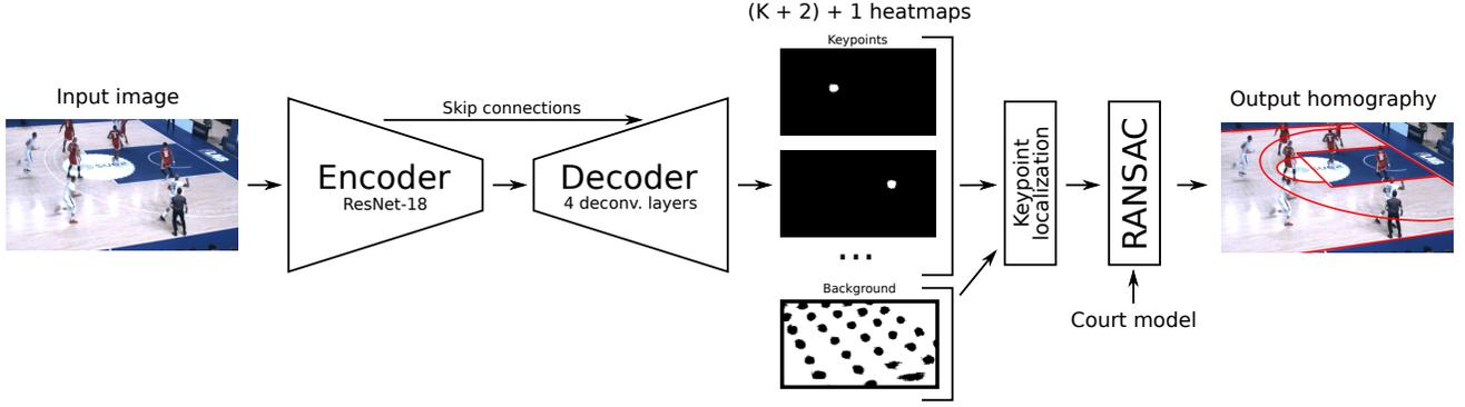
**Figure 2: Overview of KaliCalib, our sports-field registration framework during inference. An encoder-decoder network generates keypoint and background heatmaps to retrieve the keypoint positions in the image space. A RANSAC algorithm then estimates the homography between the 3D positions of the court and the 2D positions in the frame.**
