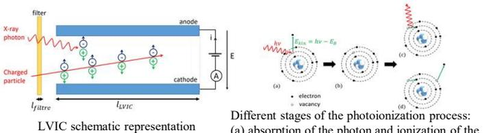
Different stages of the photoionization process: (a) absorption of the photon and ionization of the electron, (b) excited ion, (c) deexcitation through X-ray fluorescence, (d) de-excitation through Auger electron emission
