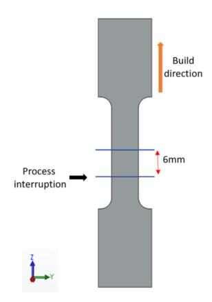
Fig. 1. Tensile tester specimen construction and process interruption
