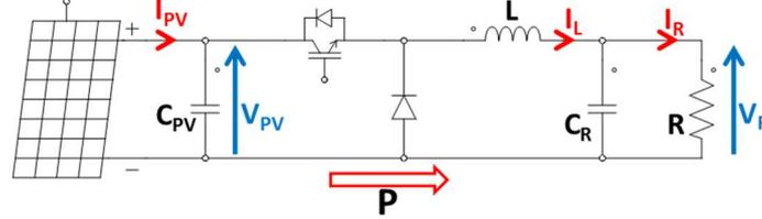
Figure 6 – Schematic of the buck chopper
