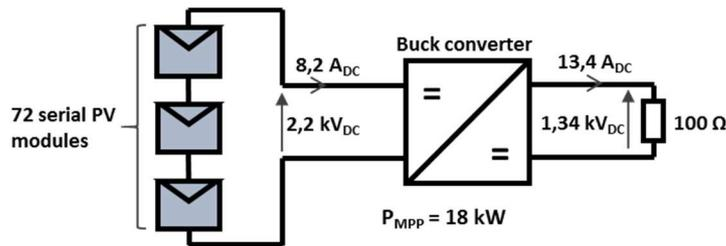
Figure 3 – General schematic of the demonstration PV plant
