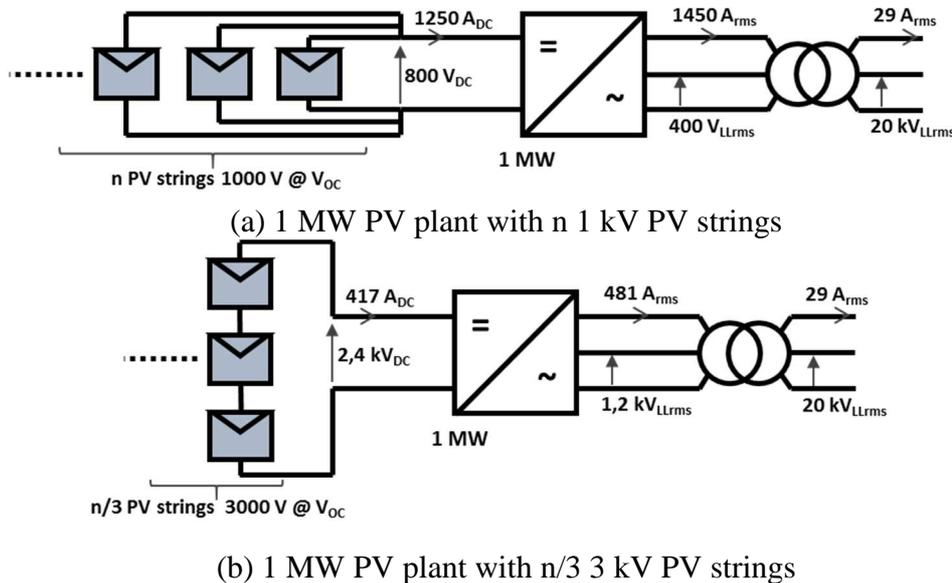
Figure 1 – Schematics comparison of a 1 kV and a 3 kV, 1 MW PV plants
