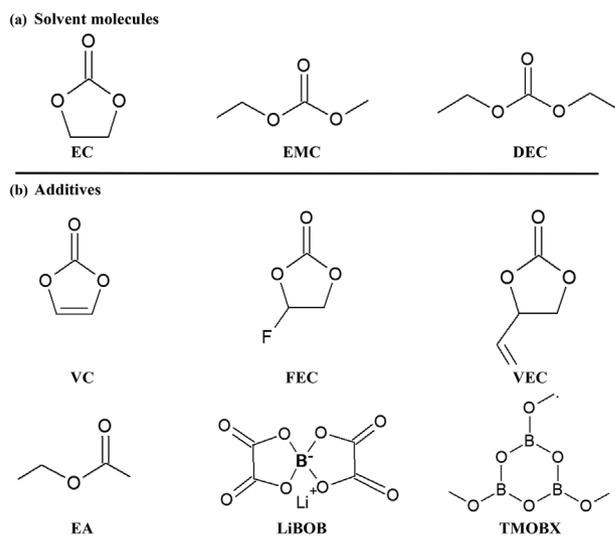
**Figure 1.** Chemical formulas of the a) solvents and b) additives used in the present work. The solvents are ethylene carbonate (EC), ethyl methyl carbonate (EMC), and diethyl carbonate (DEC). The additives are vinylene carbonate (VC), fluoroethylene carbonate (FEC), vinyl ethylene carbonate (VEC), ethyl acetate (EA), lithium bis(oxalate)borate (LiBOB), and trimethoxyboroxine (TMOBX). Salt is always lithium hexafluorophosphate at one molar concentration.
