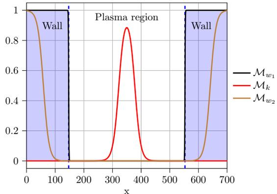
(b) The simulation domain following a magnetic field line in the SOL. Mask functions indicate whether a given point is in the wall. The wall region is shown in blue.  $\mathcal{M}_{w_1}$  is a mask describing the absorption of particles by the wall,  $\mathcal{M}_{w_2}$  is a mask describing the absorption of momentum and energy by the wall, and  $\mathcal{M}_k$  is a mask describing the kinetic source.
