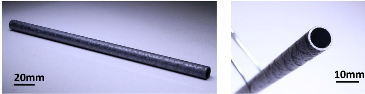
**Fig. 2.** SiC/SiC composites cladding as processed.
