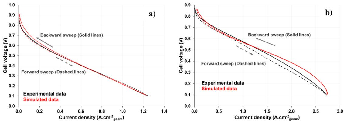
Figure 1: Comparison between experimental and simulated performances measurement: **a)** with 0.020 mg<sub>Pt</sub>.cm<sup>-2</sup> loading at the cathode **b)** with 0.1 mg<sub>Pt</sub>.cm<sup>-2</sup> loading at the cathode
