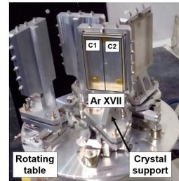
Figure 1: Top-view picture of the rotating table on which are placed the crystals sets.
