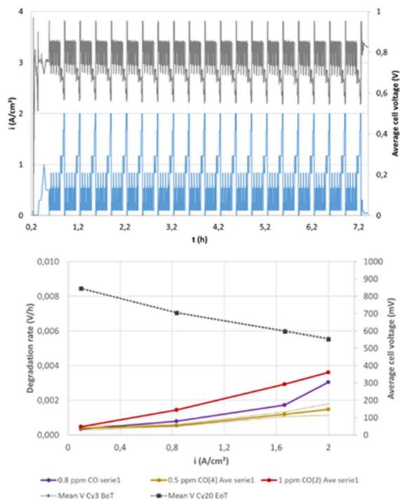
The protocols and poisoning tests under Fuel Cell Dynamic Load Cycles (FC-DLC) following Stacktest recommendations [2] are conducted over one day to better mimic operation of a car on maximum a daily period. This allowed applying 20 cycles, the two first ones being always under pure Hydrogen.
