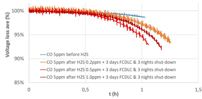
**Figure 2.** Comparison of voltage decrease in % of initial value during CO 5 ppm tolerance tests just after contamination with H<sub>2</sub>S from 0.2 ppm to 1ppm and after recovery by cycling under FC-DLC and overnight shut-downs (x3).
