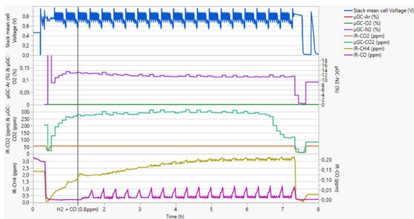
**Figure 3.** stack average cell voltage during FC-DLC and concentrations in nitrogen, argon, oxygen (in %), carbene dioxide (in ppm), methane and carbon monoxide conducted by sampling fuel from the recirculation loop.
