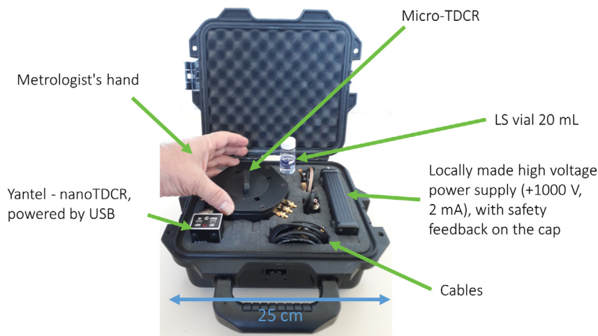
Fig. 10. The whole set of components, including locally-made high voltage supply, can be easily handled and connected to a portable computer.
