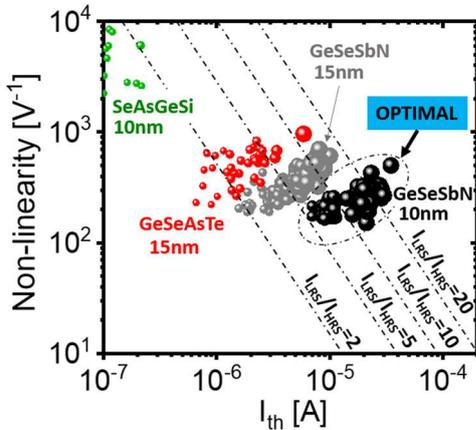
Fig. 7. Among the various OTS technologies promising durable 1S1R programming operation (**Fig.6**), the optimal 1S1R stack is extracted for 1S1R sub-threshold margin maximization. The tradeoff between OTS non-linearity and threshold currents is used for stack discretization.
