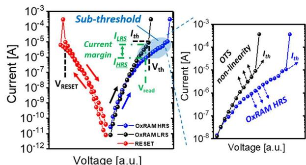
Fig. 2. 1S1R typical current-voltage characteristics. The key parameters for reliable 1S1R sub-threshold reading operation (OxRAM R<sub>HRS</sub>, OTS non-linearity and OTS threshold current) are presented. Given OxRAM R<sub>LRS</sub> << OTS R<sub>off</sub>, OxRAM R<sub>LRS</sub> impact on I<sub>LRS</sub> is considered negligible.
