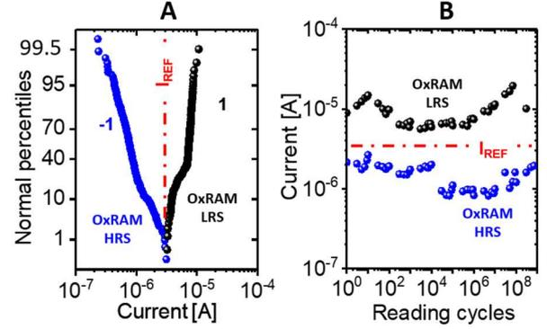
Fig. 8. A) 1S1R sub-threshold experimental cycle-to-cycle programming LRS and HRS read current distributions. Currents are extracted from five different devices. A BER  $\sim 7 \cdot 10^{-3}$  is demonstrated. B) 1S1R sub-threshold reading endurance.
