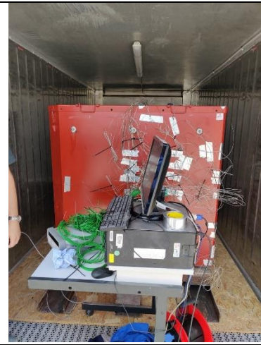
Figure 4 : Container with the external thermal sensors
