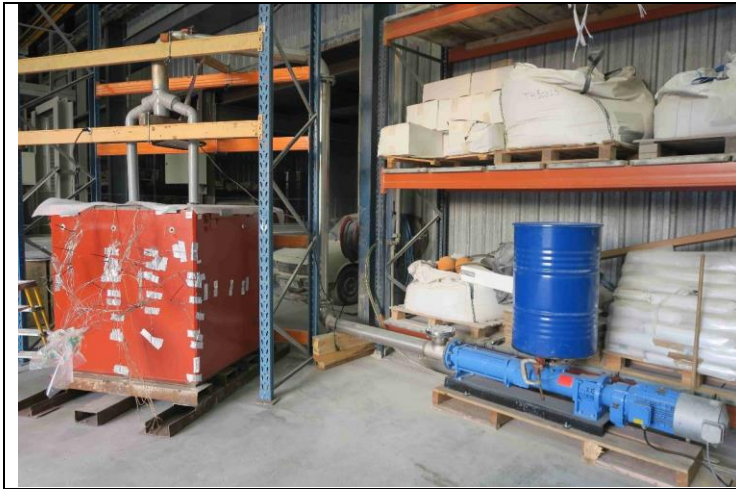
Figure 3 : Container (red) with the mortar injection apparatus
