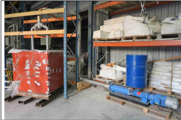
Figure 3 : Container (red) with the mortar injection apparatus
