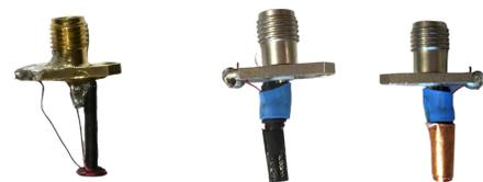
a. Radial probe b. Probes with envelopes
