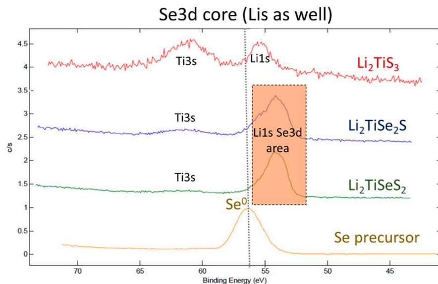
**Figure 10.** XPS spectra of powders:  $\text{Li}_2\text{TiS}_3$ ,  $\text{Li}_2\text{TiSe}_2\text{S}$ , and  $\text{Li}_2\text{TiSe}_2\text{S}$  and selenium precursor at Se3d core.
