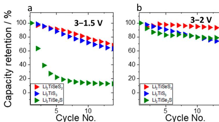
**Figure 6.** Capacity retention (%) of  $\text{Li}_2\text{TiS}_3$ ,  $\text{Li}_2\text{TiSeS}_2$ , and  $\text{Li}_2\text{TiSe}_2\text{S}$  cells cycled at a rate of  $C/10$  in different cycling windows: (a) 3–1.5 V and (b) 3–2.0 V vs.  $\text{Li}^+/\text{Li}$ .
