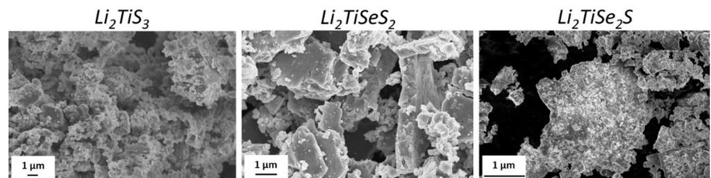
**Figure 3.** SEM images of Li<sub>2</sub>TiSe<sub>x</sub>S<sub>3-x</sub> (0 ≤ x ≤ 2) materials.
