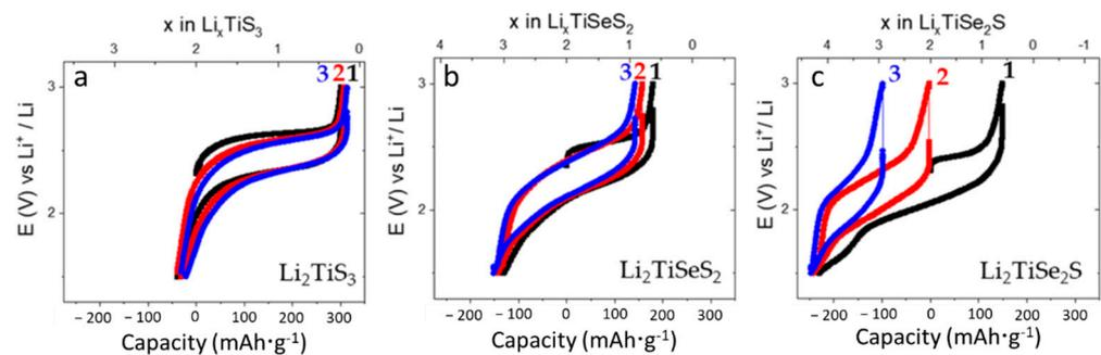
**Figure 4.** Galvanostatic curves of (a) Li<sub>x</sub>TiS<sub>3</sub>, (b) Li<sub>x</sub>TiSeS<sub>2</sub>, and (c) Li<sub>x</sub>TiSe<sub>2</sub>S cathode materials in half-cell at a rate of C/10 between 3 and 1.5 V vs. Li<sup>+</sup>/Li, the first three cycles were represented in the figures.
