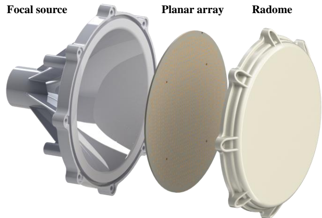
Fig. 1. Exploded view of the complete transmitarray antenna.
