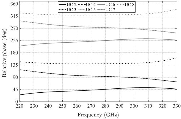
**Fig. 2.** Simulated relative phase of the transmission coefficient of the eight unit-cells, with UC 1 used as a reference. The UCs 5 – 8 comprise the mirrored design of the rotators in UCs 1 – 4, respectively, exhibiting exactly 180° phase difference. This can be seen clearly in the relative phase of UC 5, with respect to that of UC 1.
