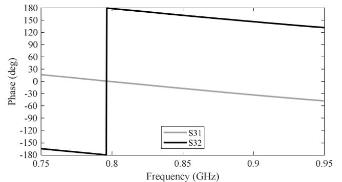
Fig. 5. Measured phase in degrees of the S-parameters of the balun, as a function of frequency.
