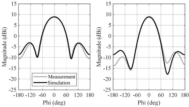
Fig. 9. Measured and simulated directivity radiation patterns of the proposed end-fire array computed on the cut-planes  $\phi = 0^\circ$  (left) and  $\phi = 90^\circ$  (right). Measurement and simulation frequencies are equal to 840 and 830 MHz, respectively. They are selected in agreement with the peak values.
