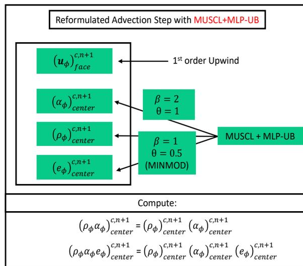
Figure 7. Reformulated advection step with the application of MUSCL+MLP-UB on primitive form of the scalars  $\Pi(\alpha_\phi, \rho_\phi, e_\phi)$ .
