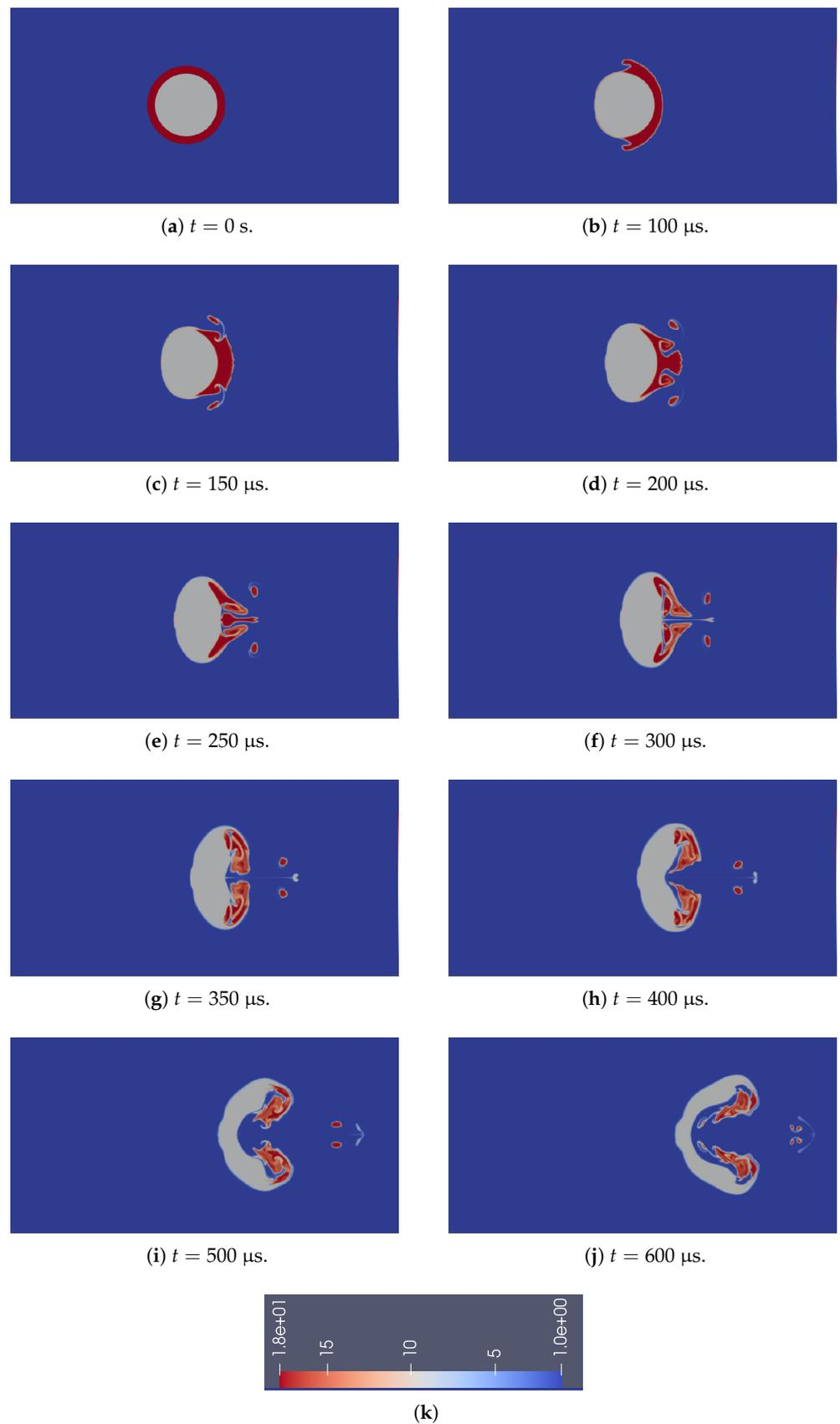
**Figure 13.** 2D numerical results for the 3-material shock-bubble interaction test case using a Cartesian mesh of size  $800 \times 400$ . Values of  $\alpha$  in *zone 3* and *zone 4* are shown together. Thus, its scale (see Figure (k)) is scaled up accordingly.
