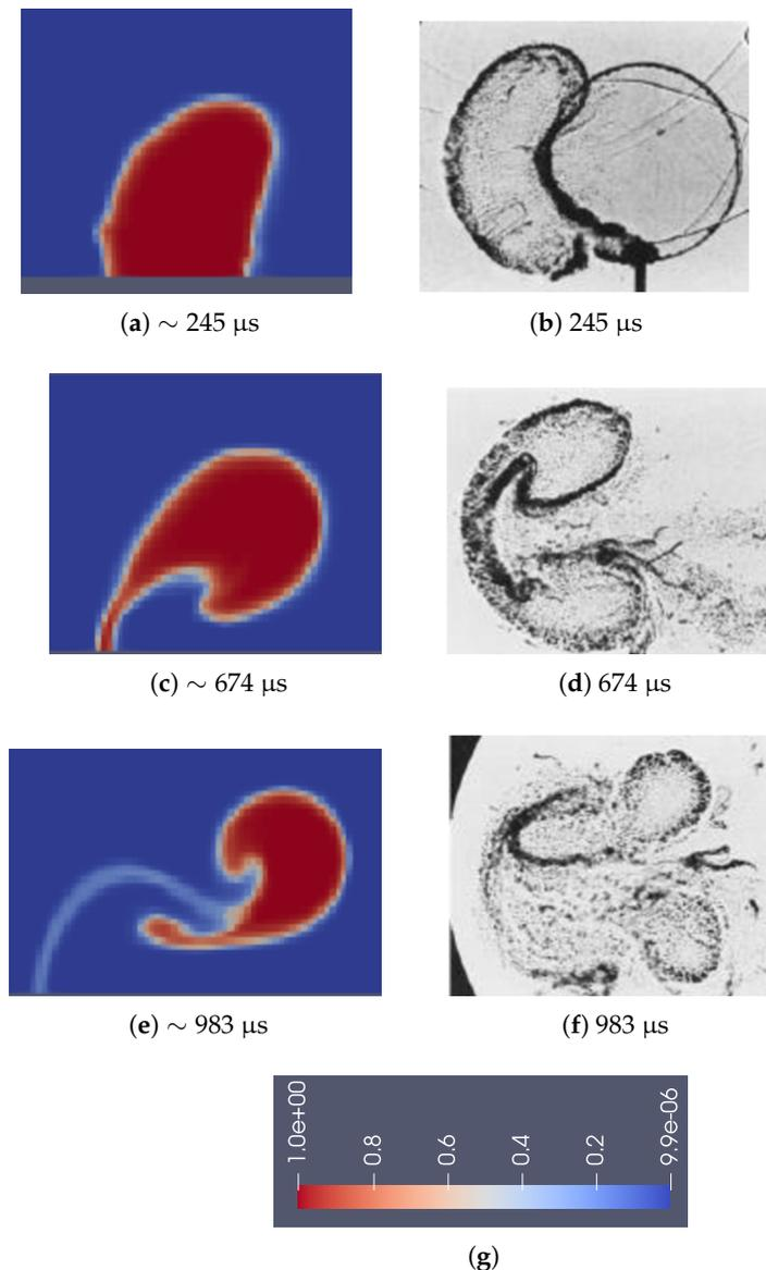
**Figure 9.** 2D numerical results for an air-helium shock-bubble interaction test case. Qualitative comparison of the cell volume fraction ( $\alpha$ ) of Helium bubble between the modeling (Figures (a,c,e)) and experimental results (Figures (b,d,f)) [47]. The scale of ( $\alpha$ ) is shown in Figure (g).
