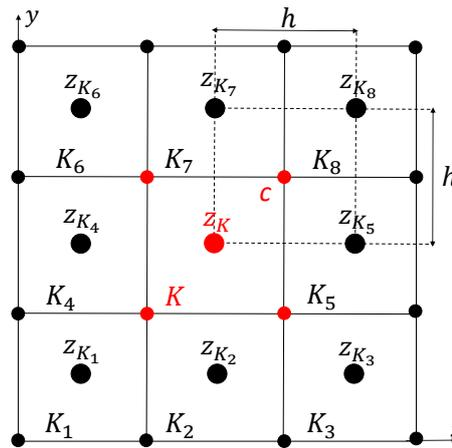
**Figure 5.** Layout of a 2D Cartesian mesh, where finite volume cells are represented by  $K$ , corners by  $c$ , value of a scalar  $z$  at cell centers by  $z_K$ , and constant distance between cell centers by  $h$ .
