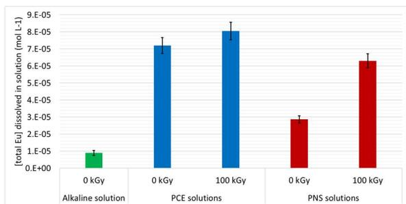
**Figure 3. Concentration of total Eu dissolved ( $\text{mol L}^{-1}$ ) in alkaline solution (without SP), PCE alkaline solutions and PNS alkaline solutions in function of dose (0 and 100 kGy) – solutions are without SP, 1 and 2 %w of PCE and PNS respectively in  $0.15 \text{ mol L}^{-1}$  NaOH,  $0.12 \text{ mol L}^{-1}$  of KOH and  $10 \text{ g L}^{-1}$  of crushed mortar (pH 13.3) –  $[\text{Eu}]_{\text{total}} = 10^{-4} \text{ mol L}^{-1}$ .**
