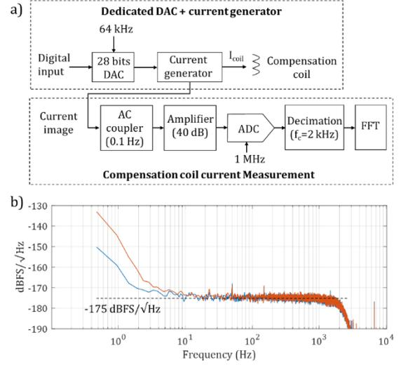
FIG. 4. Noise level performance of the compensation currents delivered by the DAC and current generator assembly in the feedback of the  $^4\text{He}$  magnetometer closed-loop architecture: characterisation method (a) and noise measurements (b). In (b) the blue spectrum corresponds to a null compensation current, and the orange one to a compensation current close to full scale, i.e. equivalent to a  $\pm 70 \mu\text{T}$  magnetic field compensation.
