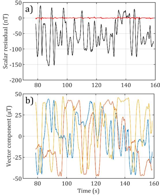
FIG. 9. Vector calibration of the  $^4\text{He}$  magnetometer. (a) Scalar residual before (black) and after calibration (red). (b) Vector components measured by the  $^4\text{He}$  OPM during the calibration process:  $B_x$  (blue),  $B_y$  (orange) and  $B_z$  (yellow).
