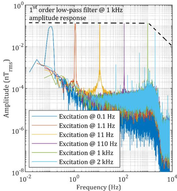
FIG. 8. Bandwidth measurement of the vector OPM operated in closed-loop configuration. Amplitude responses in  $\text{nT}_{\text{rms}}$  measured on the X axis of the magnetometer to external sinusoidal excitation with frequency ranging from 0.1 Hz up to 2 kHz. A [DC-1 kHz] bandwidth is derived from the measurements, in full agreement with the filter characteristics of the closed-loop on this axis.
