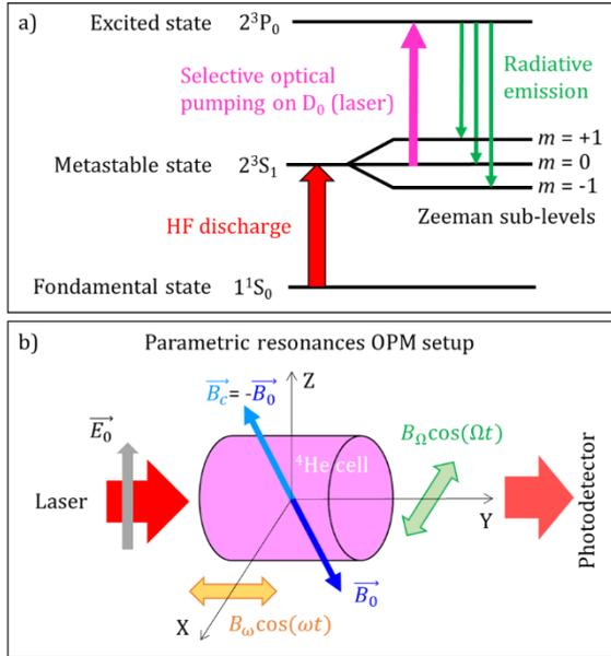
FIG. 1. (a) Simplified principle of operation of the  $^4\text{He}$  OPM: energy diagram describing the optical pumping process (b) and main elements of the parametric resonance magnetometer architecture.
