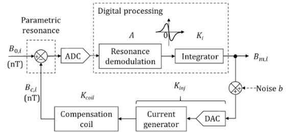
FIG. 3. Schematic of the null-field closed-loop implemented in our electronics for the compensation of the ambient vector magnetic field. In this loop,  $b$  models all types of noise sources introduced by the feedback elements as an equivalent input noise.
