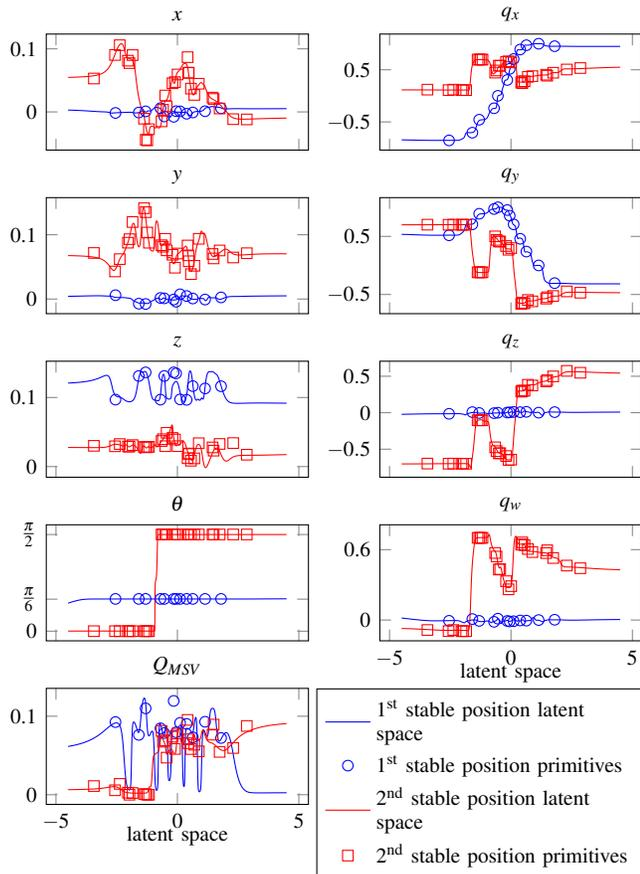
Fig. 8. QGG latent space representation for the pulley object. The curves are obtained by sampling values in  $[-4.5, 4.5]$  and passing them through the decoder. The outputs are gripper configurations stored in the latent space of the QGG. The scatter plots are obtained by passing some pulley primitive configurations through the encoder (only one third of the primitives displayed for readability).
