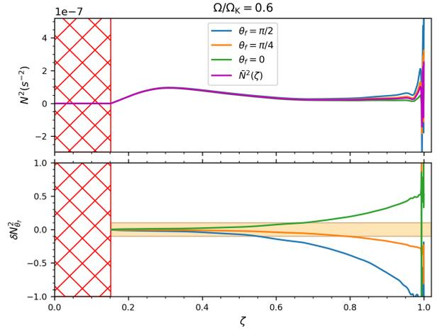
**Fig. 4.** Profile of the squared Brunt-Väisälä frequency  $N^2$  and the relative error  $\delta N_{\theta_f}^2$  of the adopted approximation (Eq. (42)) as a function of  $\zeta$  at different colatitudes  $\theta_f$  using an ESTER model rotating at 60% of the Keplerian breakup rotation rate (The light orange area indicates the margin of error which we allow and the red hatched area represents the convective region of the star).
