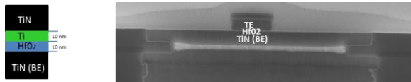
Fig. 2: Schematic Stack of the resistive memory studied (left) and SEM cross section of the stack (right).
