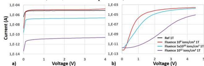
Fig. 3: Measurements carried out on single NMOS transistors (Width=660nm and Length=500nm). a)  $I_d(V_d)$  at  $V_g=1.3$  V after irradiation at three various fluences ( $10^9$  ions/cm<sup>2</sup>,  $5 \times 10^{10}$  ions/cm<sup>2</sup>,  $10^{12}$  ions/cm<sup>2</sup>) and with no irradiation (reference). b)  $I_d(V_g)$  at  $V_d=1.3$  V after irradiation (three fluences).
