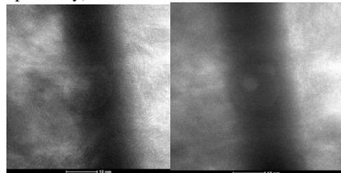
Fig. 9: TEM imaging of devices irradiated with fluence of  $10^9$  ions/cm<sup>2</sup> (left) and  $10^{12}$  ions/cm<sup>2</sup> (right).
