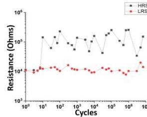
Fig. 8:  $10^7$  cycles performed on 1T 1R HfO<sub>2</sub> stack. The device was irradiated at the fluence of  $10^{12}$  ions/cm<sup>2</sup>.
