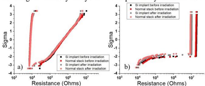
Fig. 4: LRS and HRS (a) and Pristine resistance (b) normal distribution results on two memory stacks (pure HfO<sub>2</sub> and Si-implanted HfO<sub>2</sub>) after irradiation at low fluence ( $10^9$  ions/cm<sup>2</sup>) and with no-irradiation.
