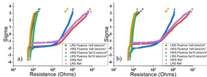
Fig. 6: Resistance distribution at the 10kth cycle for Si-implanted HfO<sub>2</sub> stack (a) and HfO<sub>2</sub> classic stack (b) with the same parameters as in Fig. 5. In the case of the classic stack, at a fluence of  $5 \times 10^{10}$  ions/cm<sup>2</sup>, V<sub>gate</sub>-set has been increased from 2.5V to 2.75V.
