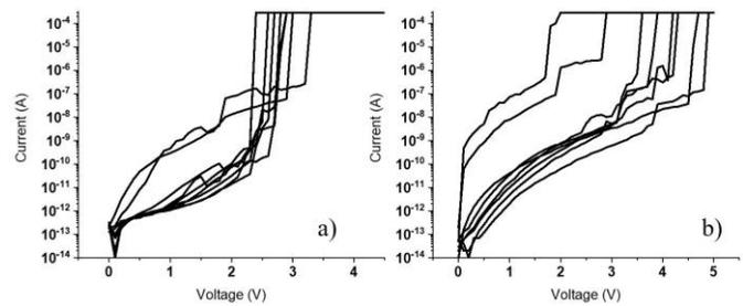
Fig. 7: Evolution of the current as function of the voltage when forming pristine OxRAM 1R devices irradiated at a fluence of  $10^9$  ions/cm<sup>2</sup> (a) and at a fluence of  $10^{12}$  ions/cm<sup>2</sup> (b).
