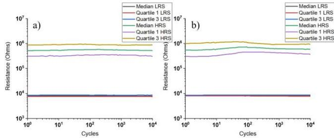
Fig. 5: 10k Cycles endurance succeeded on HfO<sub>2</sub> stack (a) and Si implanted HfO<sub>2</sub>-s tack (b) on 3072 devices after irradiation at a fluence of  $10^9$  ions/cm<sup>2</sup>.
