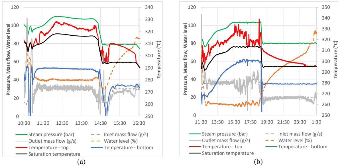
**FIGURE 4.** Pressure, mass flow, liquid level, and temperatures on water-steam side in the PCM storage section
