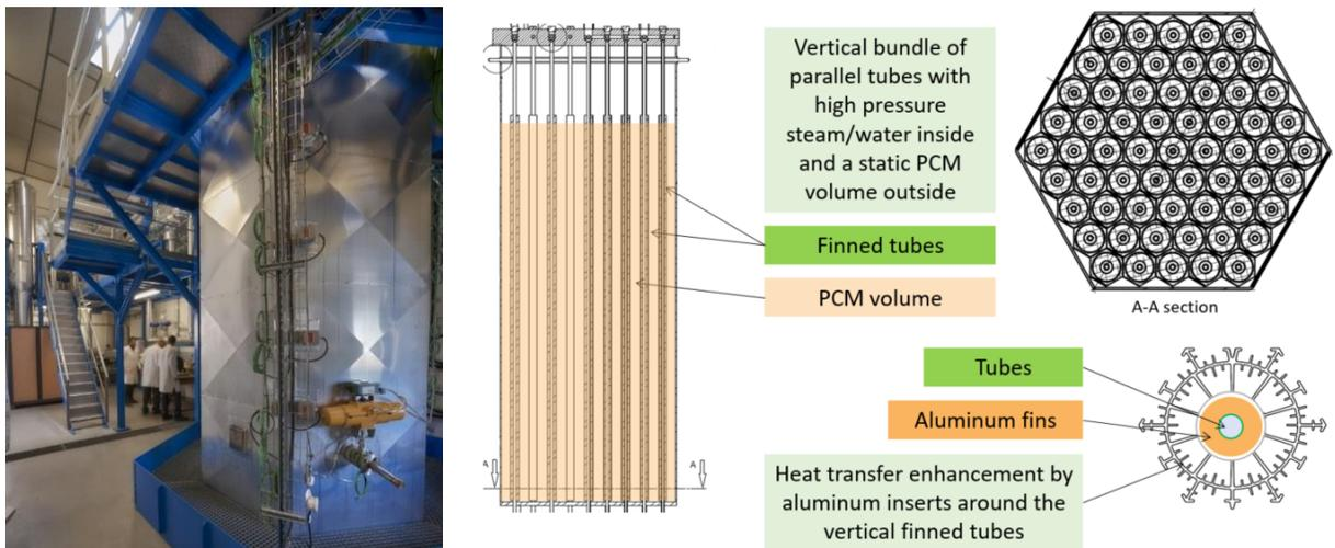
**FIGURE 1.** Picture (left) and schematic (right) of the PCM module tested during the IN-POWER project
