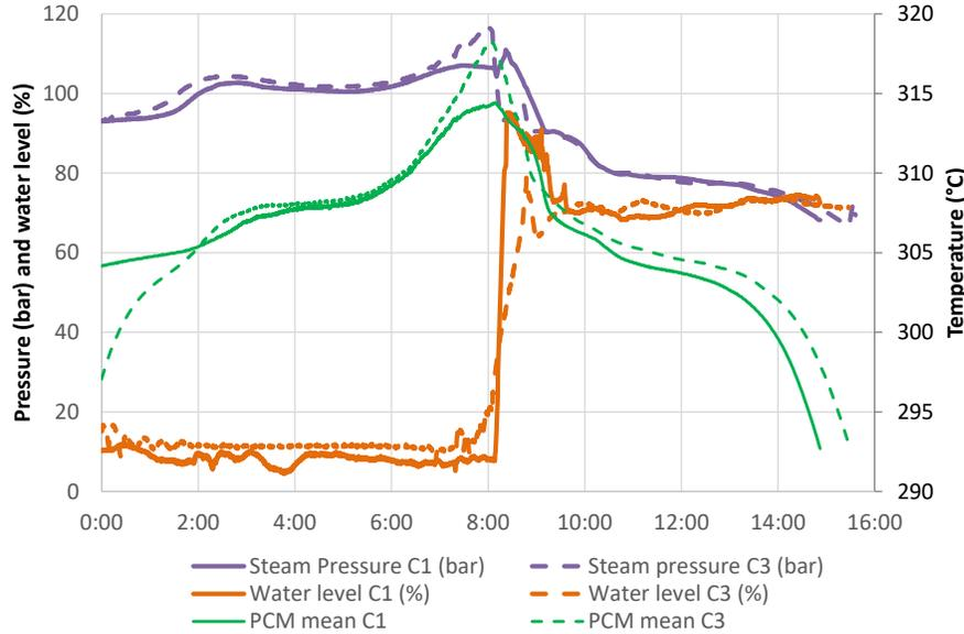
**FIGURE 2.** Steam pressure (in purple), liquid water level in the tubes (in orange), and average PCM temperature (in green) during a complete charge and discharge cycle in nominal conditions: results from the first campaign (C1) in continuous lines, results from the latest campaign (C3) in dotted lines
