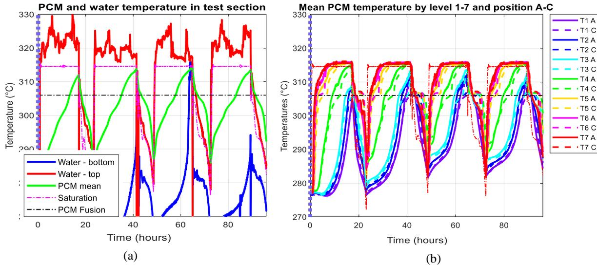
**FIGURE 3.** (a) Mean PCM and water temperatures at different locations, and (b) level-averaged PCM temperatures (T1 indicating the bottom of the tank and T7 indicating the top of the tank) during four consecutive complete charge and discharge cycles
