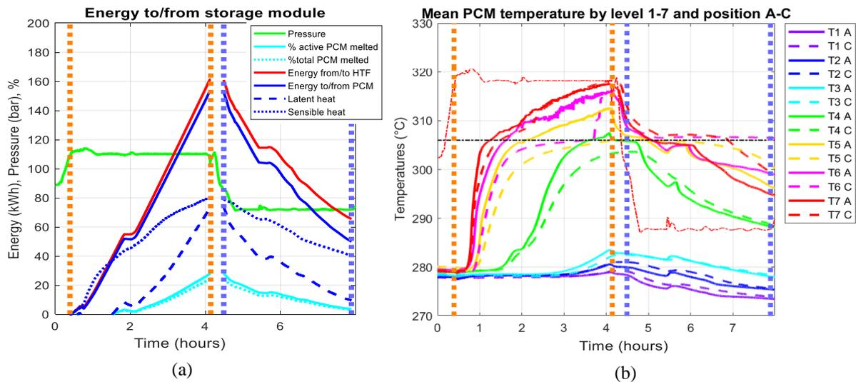
**FIGURE 5.** (a) Stored energy, PCM melted mass fraction and water pressure, and (b) level-averaged PCM temperatures (T1 indicating the bottom of the tank and T7 indicating the top of the tank) during a partial storage cycle with 30-minute flow stops in charge and in discharge. Charging periods are represented between dashed orange lines, and discharging period are represented between dashed blue lines.
