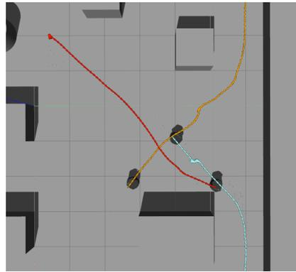
Fig. 4: Resulting trajectories example for a simulation with three robots (using LHRVO)
