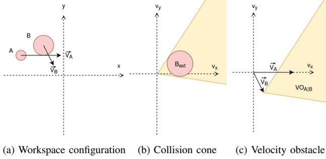
Fig. 1: Velocity obstacle faced by agent A
