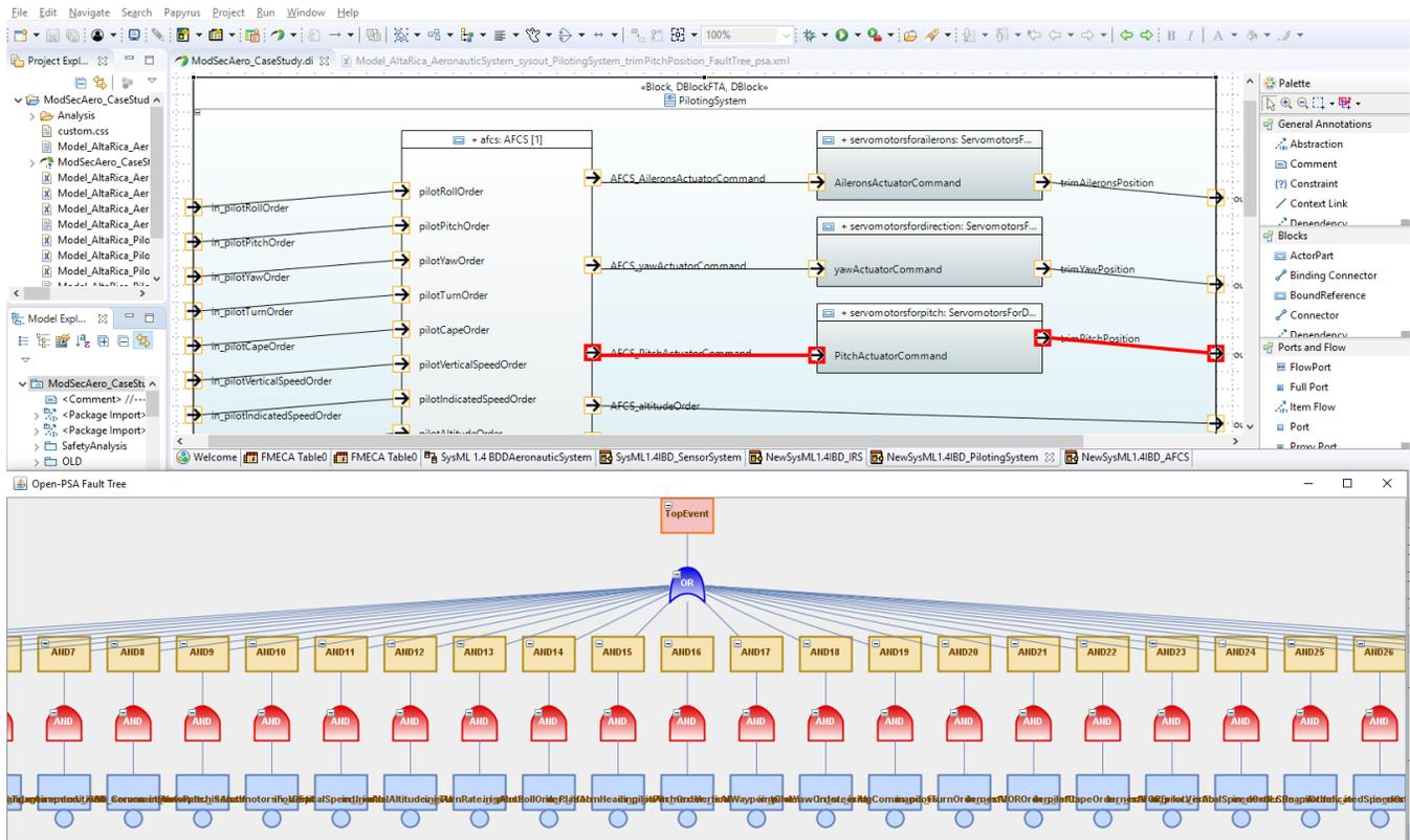
Figure 6: Overview of the attack-failure path in the FCS threat scenario and generated fault tree
